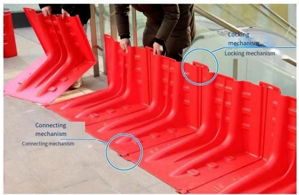
Install the flood plate from left to right, insert the connecting mechanism first, and then fasten the locking mechanism. If you need to adjust the Angle, you can use the locking mechanism to fine tune the placement Angle  $\pm 3$ .
